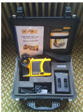
Figure 2. Apparatus of the National Centre - Thermovision camera
