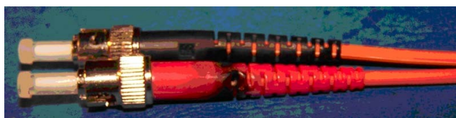
Figure 5. Damaged terminals of optical cables
