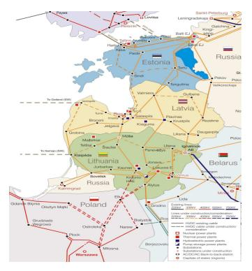
Fig.1. The map of the interconnection solutions for the Baltic States
