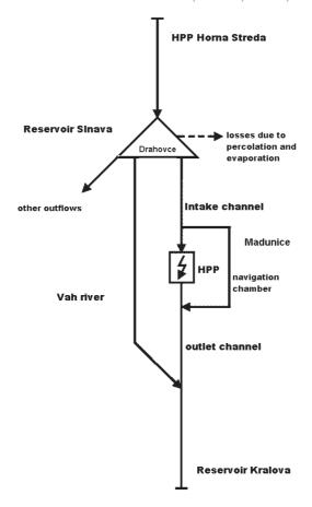
Fig.1 Scheme of water work Drahovce - Madunice
