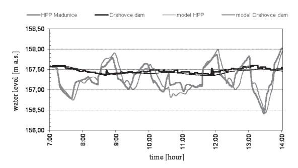
Fig. 4 Comparing water level measurements to results from model
