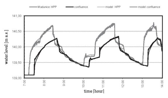
Fig. 3 Comparing water level measurements to results from model
