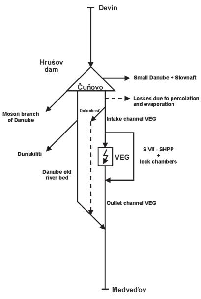
Fig. 4 Scheme of water work Gabcikovo
