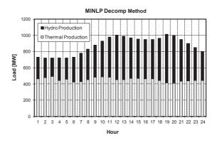
Figure 3. Power generation from hydro and thermal plants.
