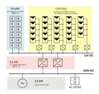
Fig.5 Scheme of the proposed hybrid system.
