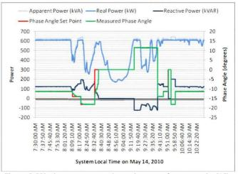
Figure 5: PV plant response to change in power factor set point [15]
