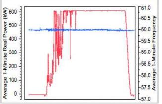
Figure 6: PV plant power output (red) and grid frequency (blue) on April 11, 2010 [15]
