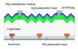
Figure 2 Cell structure with boron-diffused front emitter [16]
